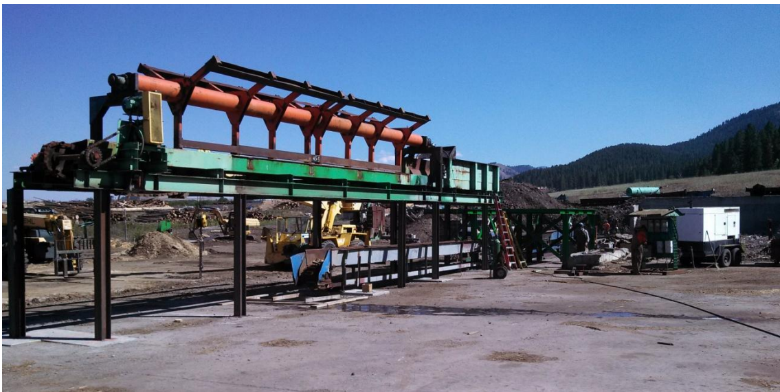
The new mechanized log sorting line at Integrated Biomass Resource in Wallowa, Ore. Funds from ODF helped the facility secure a $3.4mil loan to purchase the new equipment and add 15 new jobs. Photo: Nils Christoffersen, Wallowa Resources
